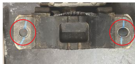
Figure 1: Swaged bolt holes to be drilled
