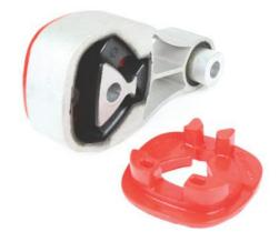
Figure 1 - Fit Inserts into voids.
